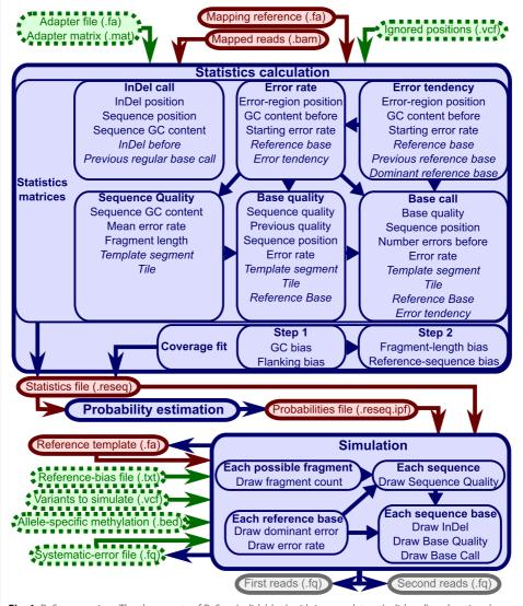
**Fig. 1** ReSeq overview. The three parts of ReSeq (solid, blue) with its mandatory (solid, red) and optional (dotted, green) inputs. The italic entries for the statistics matrices are independent dimensions in the matrix, while the normal entries are reduced to two-dimensional interactions
